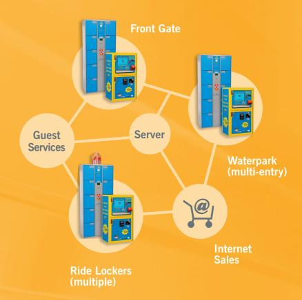
**How it works:** Locker Link wirelessly networks all of the lockers, wristband dispensing kiosks, and manned POS in your facility. Individual guests and groups can jump from locker to locker throughout the day for a single price.
